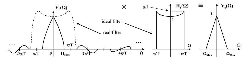
which means the output of  $h_r(t)$  is also given by:  $y_c(t) = \sum_{n=-\infty}^{\infty} x_c(nT) \frac{\sin \pi (t - nT)/T}{\pi (t - nT)/T}$ as we have already concluded before.
