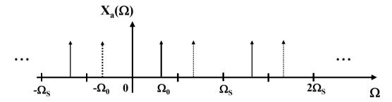
recovered signal after low-pass filtering, with cut-off at  $\Omega_S/2: x_c(t) = \cos(\Omega_0 t)$
