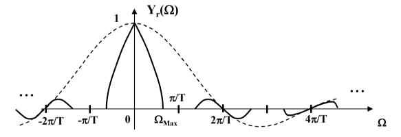
from where it can be concluded that the zero-order reconstruction distorts the  $Y(e^{j\Omega T})$  spectrum in a way that can be compensated for, if we consider the base-band replica which is the one we want to recover; in addition, all other replicas which we want to eliminate, are strongly attenuated which alleviates the filtering effort of  $h_r(t)$ .
