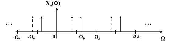
recovered signal after low-pass filtering, with cut-off at  $\Omega_S/2: x_c(t) = \cos[(\Omega_S - \Omega_0)t]$
