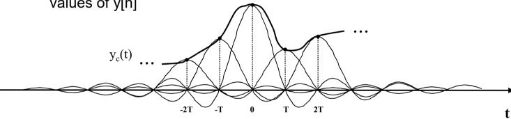
using frequency-domain analysis, and considering y[n]=x[n] which implies:  $Y_a(\Omega) = Y(e^{j\omega})_{\alpha=\Omega^T} = X(e^{j\omega})_{\alpha=\Omega^T} = X_a(\Omega)$
