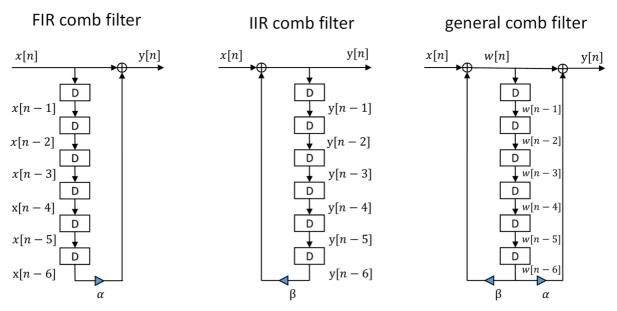
Using the Z-Transform and its properties, and assuming causality, it can be easily shown that the transfer function of the illustrated FIR comb filter is
