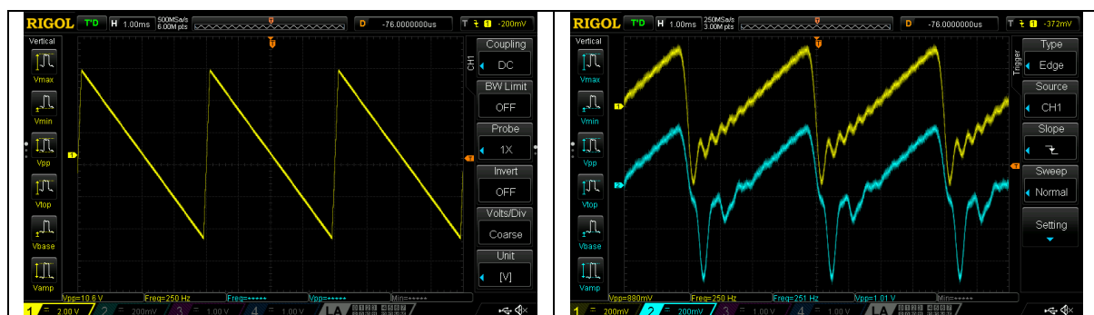
Figure 2: Left: input sawtooth wave (5 Vpp, 250 Hz, 5% Duty cycle). Right: R LINE OUT signal when y[n]=x[n] (yellow color), and L LINE OUT signal and when the 2 nd -order All-Pass system is used (with r=0.8 ).
