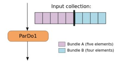
$\label{eq:parallelism} Parallelism \mbox{ within transform: when the ParDo executes, workers can process bundles in parallel}$
