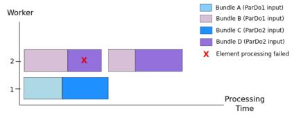
Notice that keeping bundles A-C, B-D in the same worker makes the processing more efficient.
